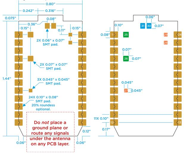
In addition to the 24 pins around the outside of the Photon, there are 7 pads on the bottom the Photon PCB that can be used to connect to extra signals: RGB LED outputs, SETUP button, SMPS enable line and USB D+/D-. Photon Pins #25-31 are described in the <u>Pin out diagrams</u>. Solder mask around exposed copper pads should be 0.1mm (4 mils) larger in all directions. E.g., a 0.08" x 0.10" pad would have a 0.088" x 0.108" solder mask.
